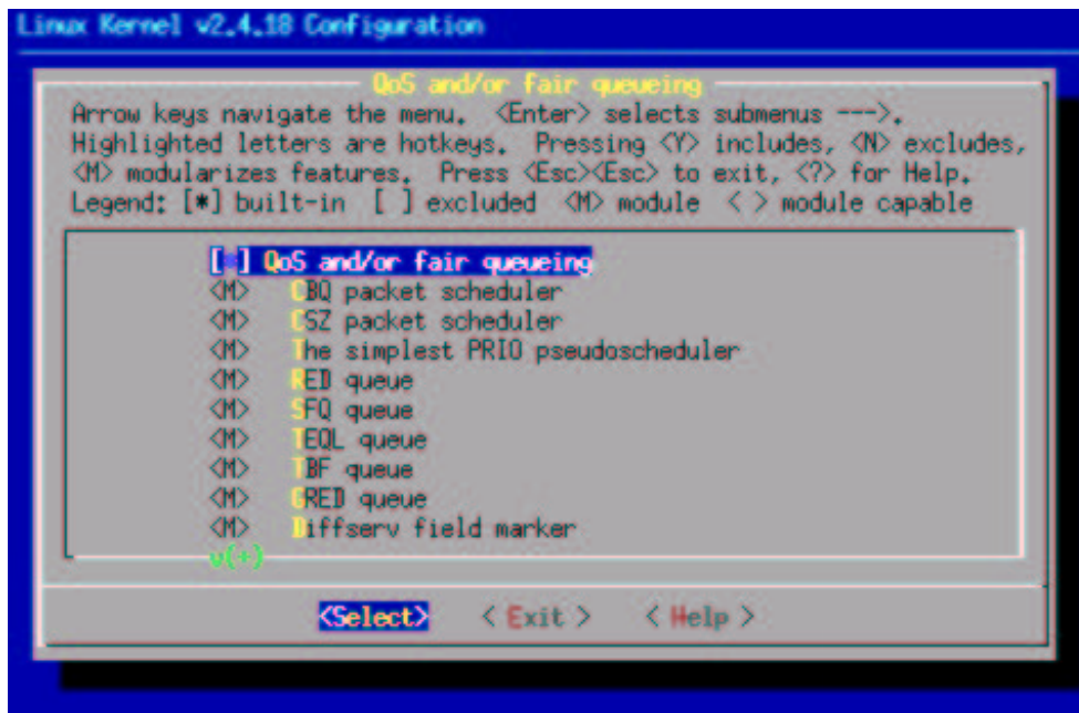
Figure 3: The 'QoS and/or fair queueing option under 'Networking Options' in the Linux kernel configuration
